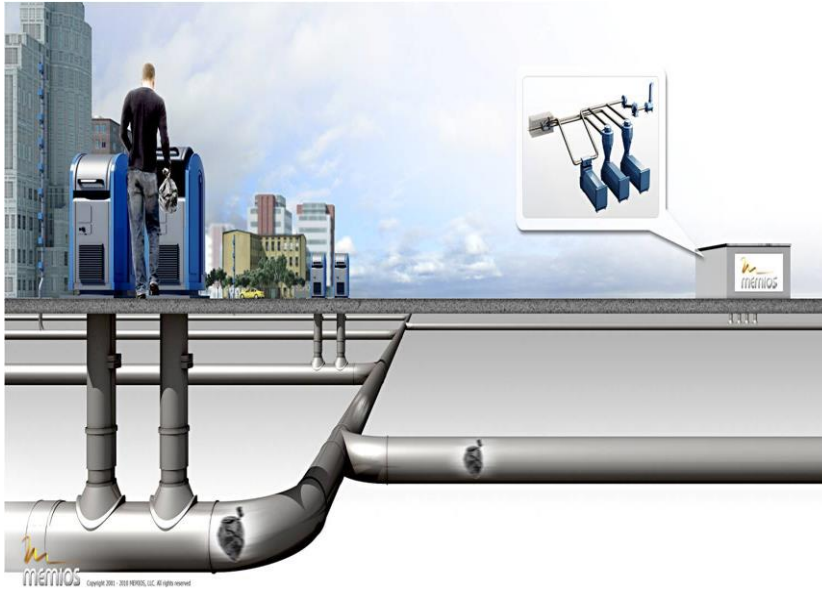
MODERN PLUMBING SYSTEM FOR TRASH AND RECYCLABLES
